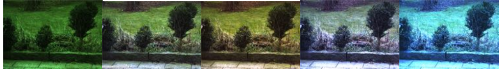
Fig. 5-31: Colour transformation OFF, D50, D65, TL84, A
