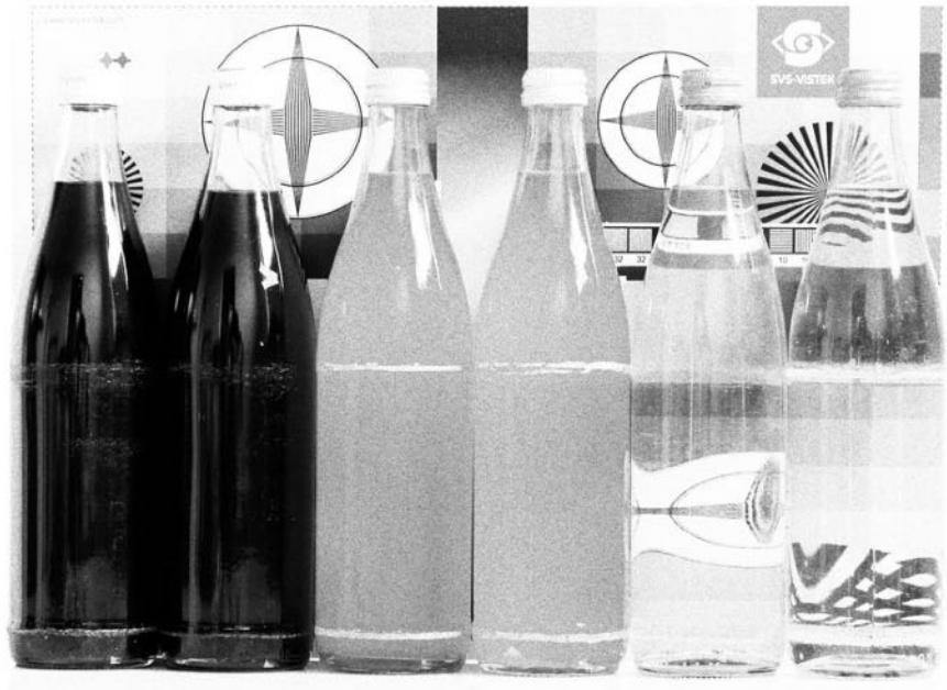
Fig. 5-1: Noise caused by too much gain
