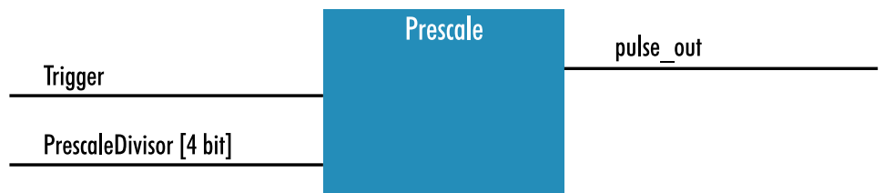
Fig. 5-48: The prescale module
