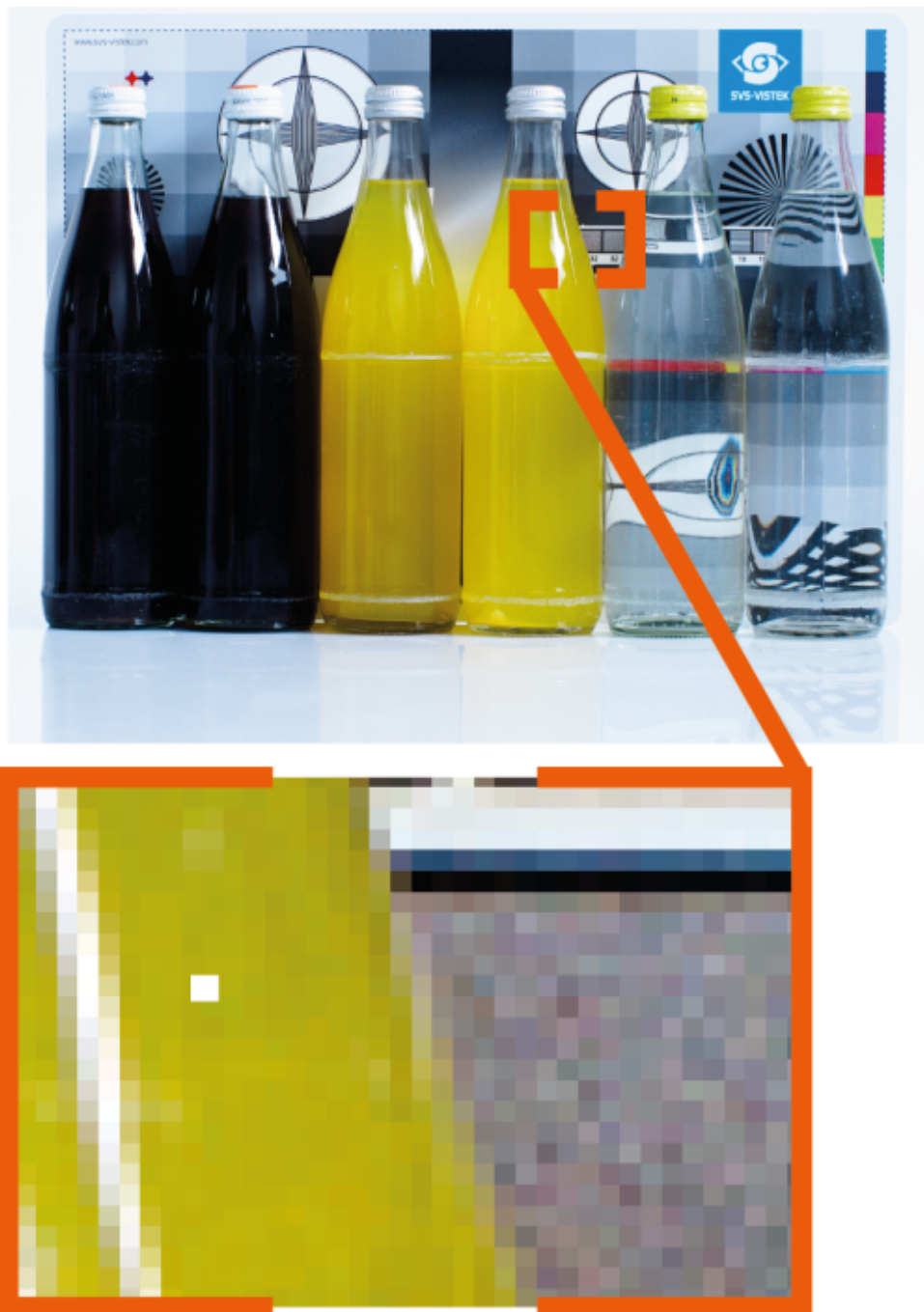
Fig. 5-23: Illustration of a defect pixel
